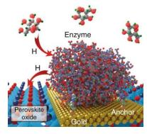
detected at concentrations of 5•10<sup>-17</sup> M. A similar device was built for sensing glucose molecules by linking a glucose oxidase enzyme to the perovskite nickelate lattice (rather than HRP). This device was selective enough to respond only to glucose and not to mannose or galactose. It could detect glucose at concentrations of 5•10<sup>-16</sup> M.
