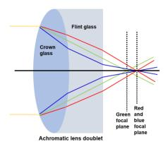
resulting from the crown glass and flint glass cancel each other out, correcting for chromatic aberrations in two wavelengths and creating a single focal plane for both of these wavelengths of light. In addition, achromatic objectives correct for spherical aberrations in a single wavelength which lies between two chromatically corrected wavelengths.
