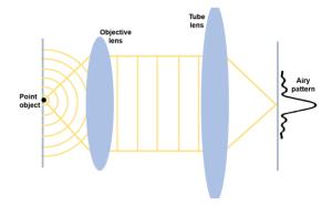
wave. Part of this spherical wave is converted into a plane wave by the objective lens. Next, the tube lens focuses this light. At the focus on the image plane, the waves constructively interfere since they exhibit the same optical pathlength. But around this point, the optical pathlengths are different and a series of concentric circles of destructive and constructive interference occur. This phenomenon is called the Airy pattern.
