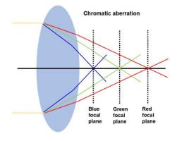
Unfortunately, light refracts at different angles towards the edges of these kinds of lenses. This is a result of the angle of incidence for parallel rays changing with the increasing curvature near the edges. With different angles of refraction, distinct focal planes occur, producing lens aberrations called spherical aberrations.
