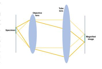
$$M = \frac{f_{\text{tube}}}{f_{\text{objective}}}$$
