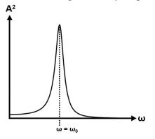
Resonance can be further characterized by computing the maximum amplitude  $A_{max}$  of oscillations where  $\omega = \omega_0$ . This quantity is given by the following equation.
